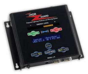
**Background:** A THOR GUARD Lightning Prediction System looks at the electrostatic "charge" of the atmosphere to determine when conditions are favorable for lightning to occur. In order to have a lightning strike in your area, there must be a "build-up" of the electrostatic field. A THOR GUARD Lightning Prediction System has the following basic components:
