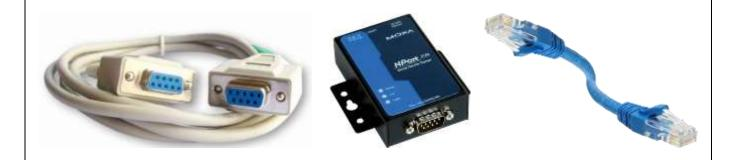
This setup is a bit more complex using a Serial to Serial cable connecting the Thor Guard unit to a MOXA Data Forwarding Device. The MOXA Data Forwarding Device then connects, using an Ethernet cable, to either your Network or the Internet in order to forward your Thor Guard data to your ThorPCX computer. For more information or to order a MOXA Data Forwarding Device, go to the MOXA Website:
